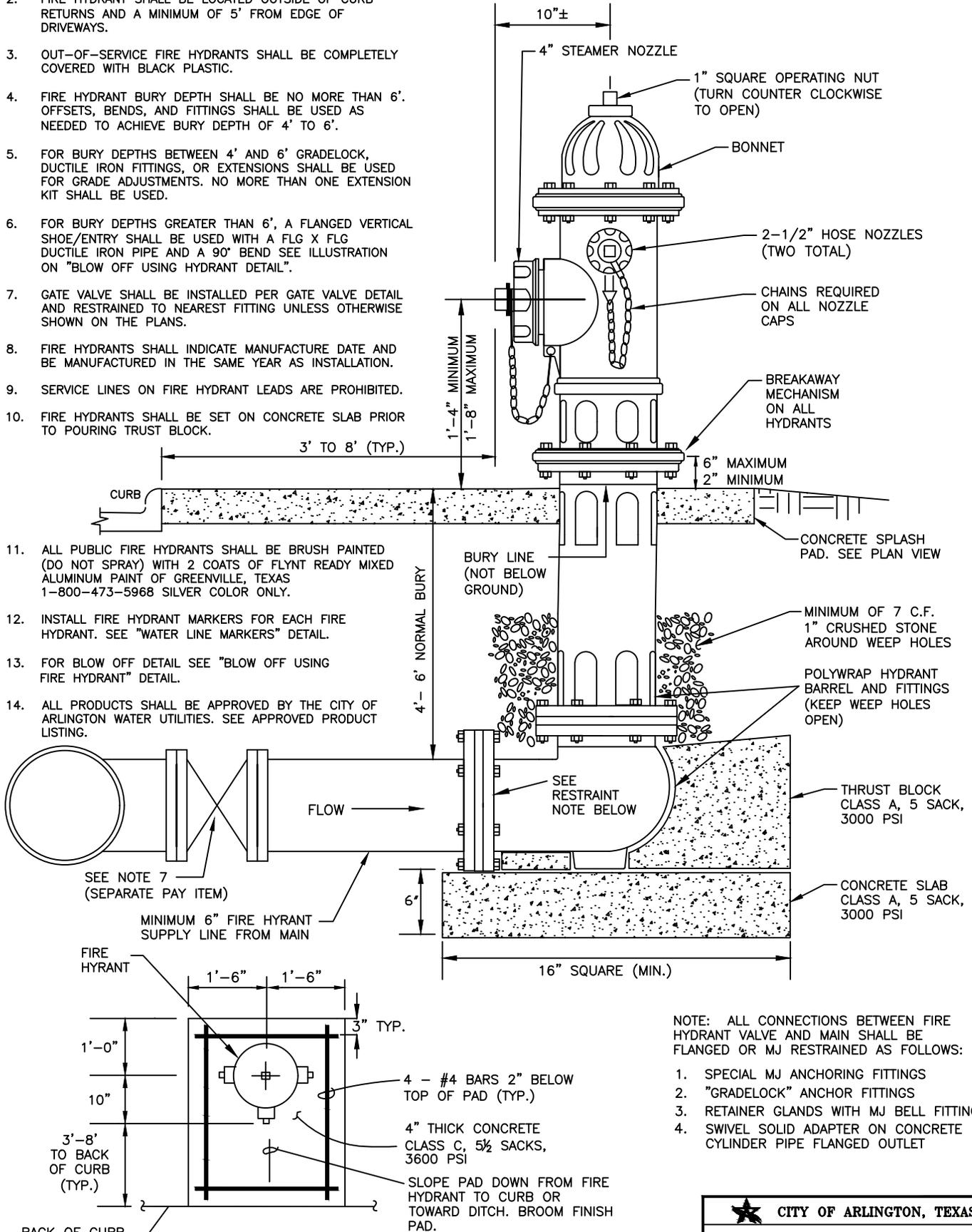
NOTE: ALL CONNECTIONS BETWEEN FIRE HYDRANT VALVE AND MAIN SHALL BE FLANGED OR MJ RESTRAINED AS FOLLOWS:
