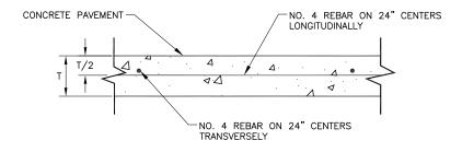
PAVEMENT REINFORCING NTS REV: 8/8/17
