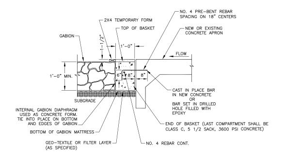
GABION TO CONCRETE ATTACHMENT NTS REV: 7/11/17
